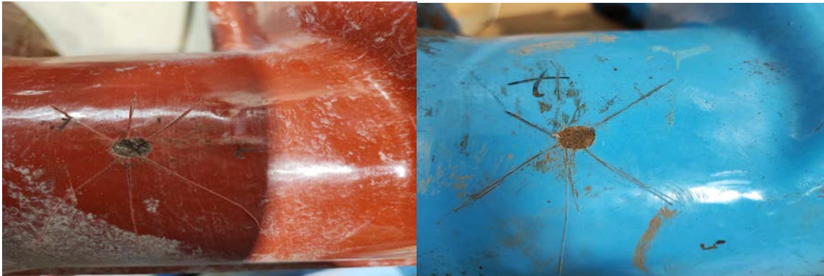
Close-up of the artificial defect: no corrosion or delamination visible
