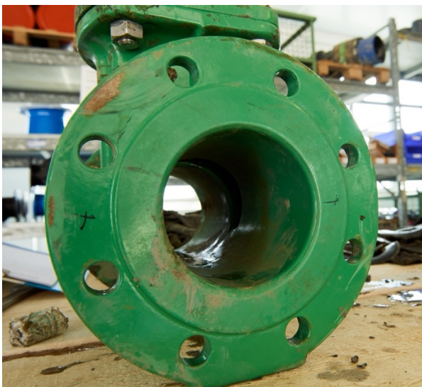
Close-up of a gate valve immediately after removal: no corrosion visible on the inside surface.
