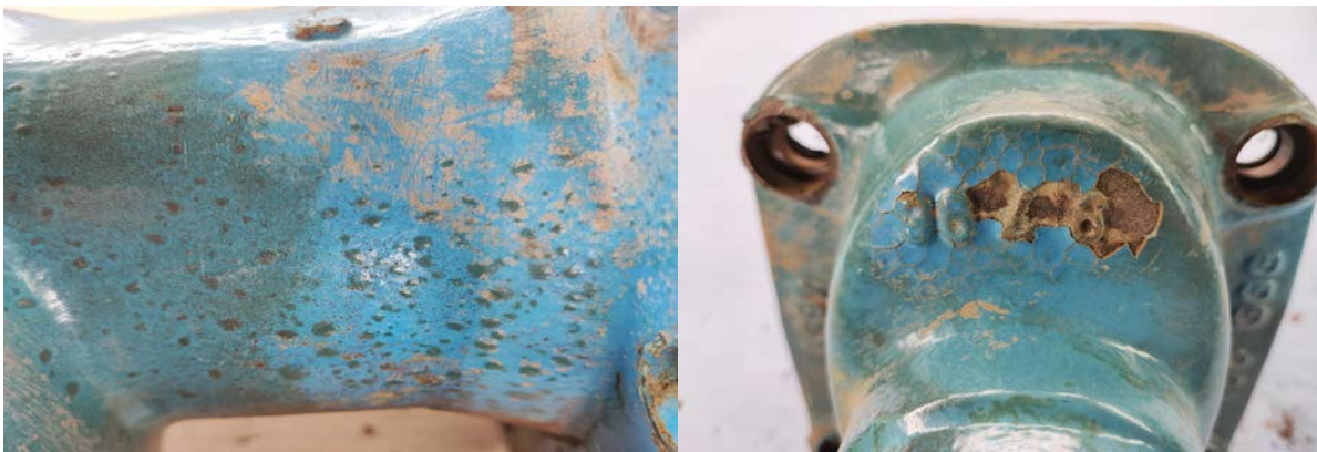
Blistering on the gate valve body; cracking and corrosion on the outer coating of the cap
